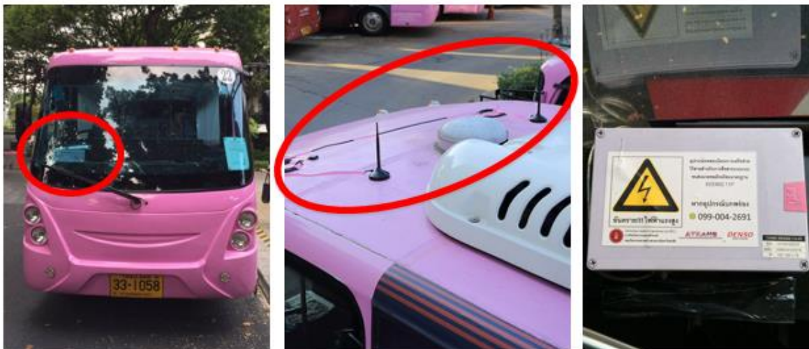
Figure 10. Testing Device Installation on Shuttle Bus.
